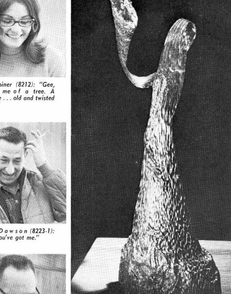
WHAT IS IT? One end of a nearly dissolved copper anode (positive electrode) after spending three years in an acid sulfate solution electroplating materials.
